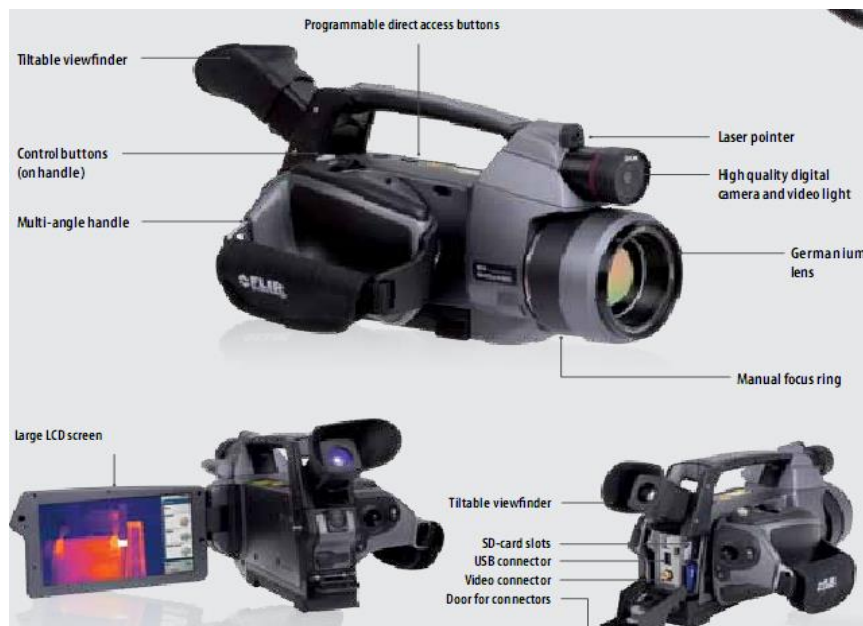
Fig. 1. The component elements for Thermo Camera Flir SC640 [2,3,4]
