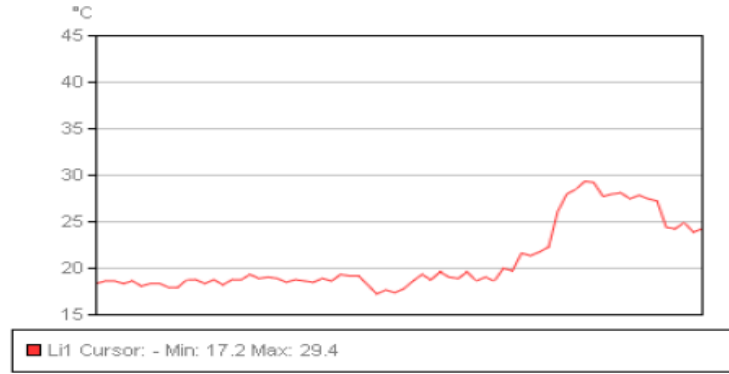
Fig. 4. Variations of the needle temperature at 300 sinkings/min.
